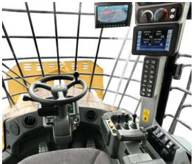
Improving operator efficiency remains a key design goal for the 950M and 962M. Ensuring operators are safe, confident in the control of their machines, have a clean, comfortable and quiet operating environment with controls that are intuitive and low effort all contribute to lower operator fatigue and better performance.
