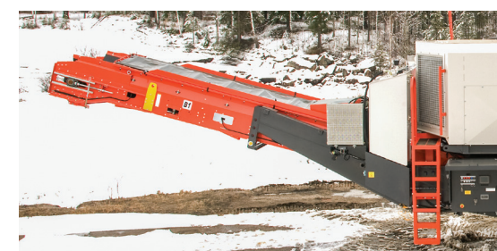
Dust-sealed, wide main conveyor
