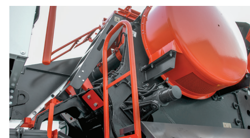
CJ412 jaw with hydraulically adjustable CSS
