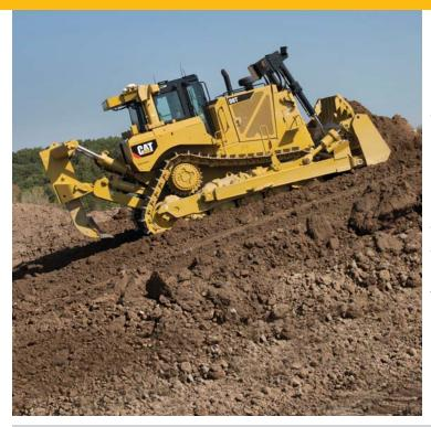
The D8T is built on a tough mainframe designed to absorb high impact shock loads and twisting forces. A fully suspended undercarriage provides more ground contact, especially in hard, uneven terrain. Greater traction means less slippage, better balance and a smoother ride.
