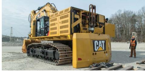
Positive Pin Retention 2 (PPR2) prevents looseness of the track pin in the track link, reduces stress concentrations, and eliminates pin walking for increased service life.
