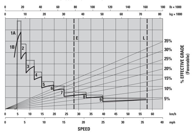
1A – 1st Gear (Converter Drive)
