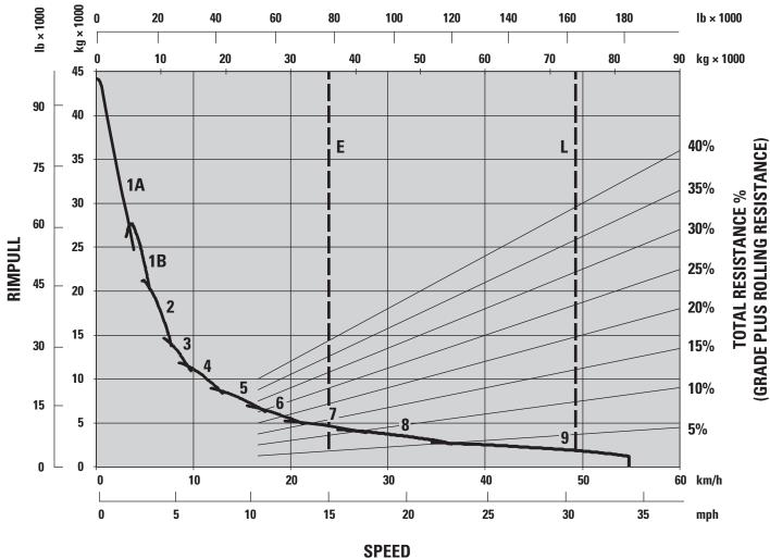
1A – 1st Gear (Converter Drive)
