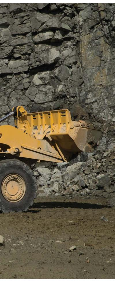
While the electric drive transmission replacement on the 988K enables the significant increase in efficiency, the axles and the driveline are the same as on the proven 988K mechanical drive.
