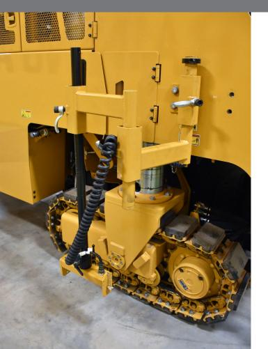
Each sensor has five transducers; the high and low readings are discarded and the remaining three are averaged for a true average reading.
