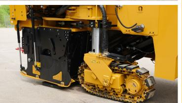
The right rear leg articulates, a feature that allows it to be positioned outboard of the cutting chamber for maximum stability and traction in demanding cuts, or inboard in front of the rotor chamber for enhanced flush cutting capability.
