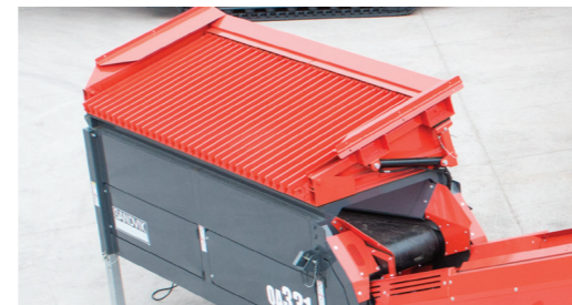
Hopper complete with hydraulic tipping grid
