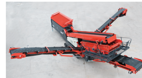
Three discharge conveyors
