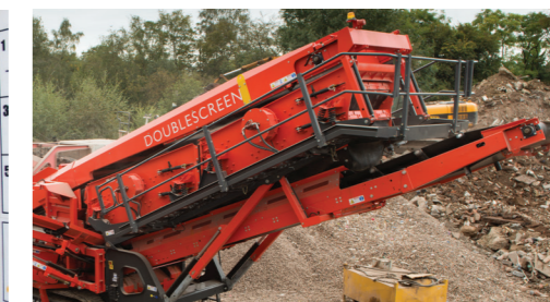
Hydraulically folding walkways for ease of maintenance
