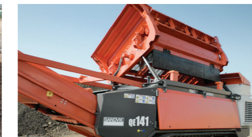
Tipping function activated by radio remote control
