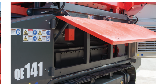
Hydraulically folding doors for easy access
