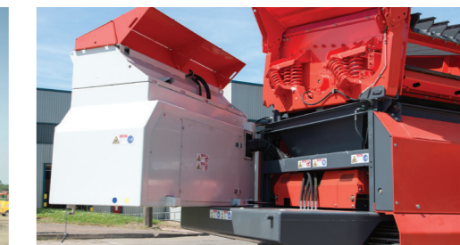
Hydraulically opening powerpack for ease of maintenance
